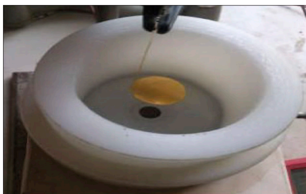
Figure 4. Show the electrochemical etching method
