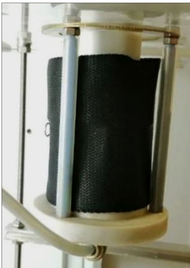
Figure 6. Accessories for fastening the processed material Busofit in an electric pulse installation
