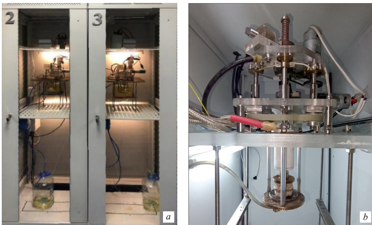
Figure 4. Electric pulse plant for the production and deposition of metal nanoparticles ( a ) and its reactor ( b )
