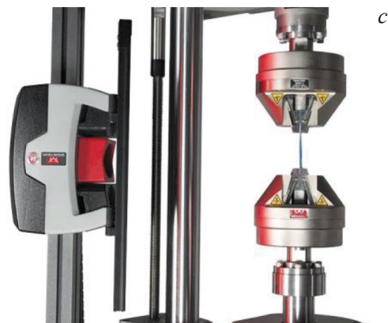
Figure 2. The typical setup for Instron tensile tester as given by: (a) in [41]; (b) in [41]; and (c) in [44]
